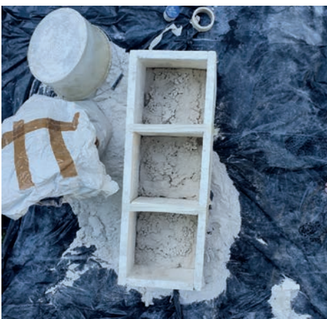
stripping the final plaster material from it's cast
