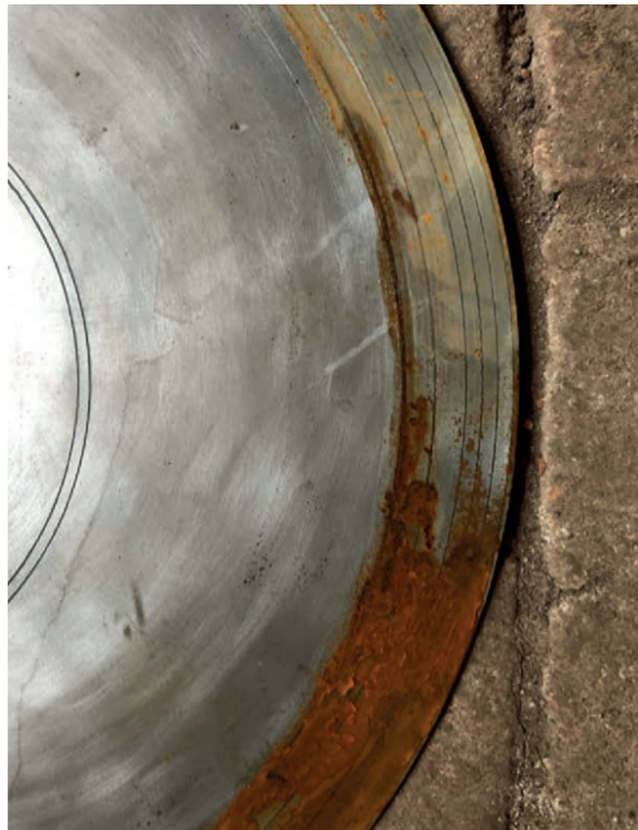
steel plate before and after corrosion
